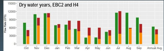
Figure 6c. Simulated average monthly pumping totals (in cfs) during 1979 (below normal water year) under the existing condition scenario (EBC2) and scenario H4.
